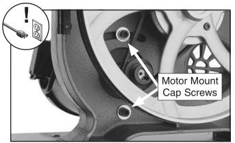
Figure 45. Motor mount cap screws.
